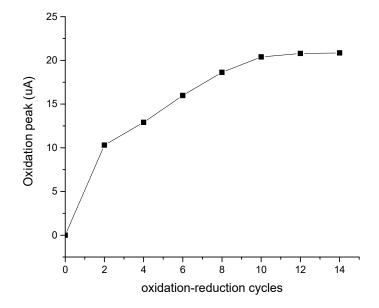
**Figure 6.** The oxidation peak currents at 530 mV were plotted against the scanning cycles. It can be seen that the oxidation peak current increases with the number of scanning cycles. The increment gradually reduces, and when the voltammetry redox scan reaches a certain amount of cycles (in this case around 10 cycles), the oxidation peaks reach a plateau state.
