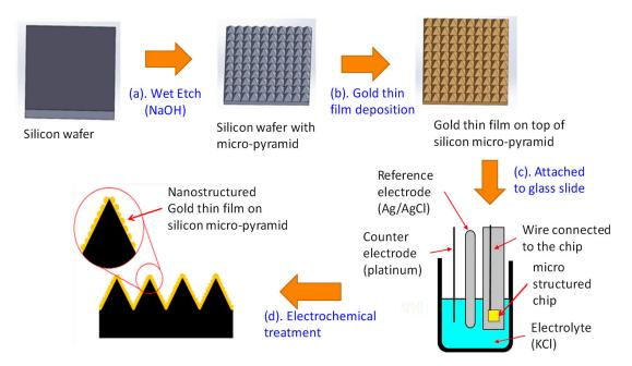
**Figure 1.** The fabrication process of the described micro/nano hierarchical structure. (**a**) The silicon wafer was wet etched in a mixed solution of NaOH, water, and isopropyl alcohol. (**b**) Depositing a gold thin film on the micro-pyramid array using a sputtering system. (**c**) Attach the chip to a slide before electrochemical treatment. (**d**) The sample was treated with electrochemical oxidation and reduction cycles to create nanostructures on the surface of the gold thin film.
