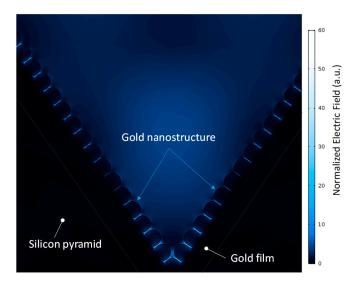
**Figure 8.** A cross-sectional view of the electric field distribution between two micro-pyramids with an incident light wavelength of 633 nm. In this figure, the normalized electric field represents the ratio between the electric Field excited by the local surface plasmon resonance and the background electric field.
