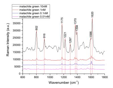
**Figure 10.** The figure shows measured SERS spectra for malachite green concentrations ranging from 0.01 nM to 10 nM on SERS substrates.
