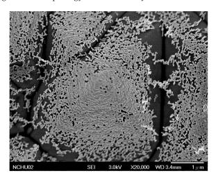
**Figure 4.** The gold film on the surface of the pyramid is oxidized and corroded. After too many oxidization-reduction cycles, the gold film became too thin and exposed the pyramid.
