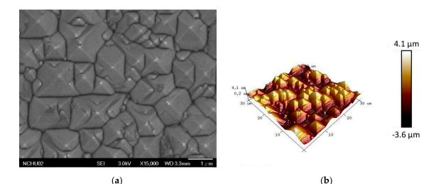
**Figure 2.** (a) The SEM image of pyramid microstructure formed by anisotropic wet etching. (b) The pyramid size measured by an atomic force microscope (AFM), the overall pyramid average height is 2  $\mu$ m, and the average spacing is 2.8  $\mu$ m.
