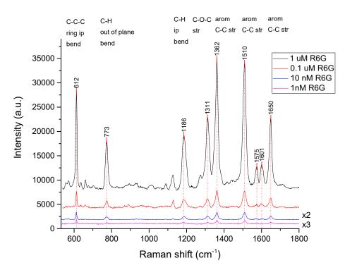
**Figure 9.** Shows the SERS spectra of R6G solutions with concentrations of  $1 \times 10^{-6}$  M,  $1 \times 10^{-7}$  M,  $1 \times 10^{-8}$  M, and  $1 \times 10^{-9}$  M, respectively, using our SERS substrate with 10 oxidation-reduction cycles.
