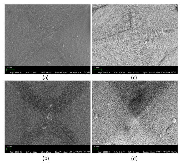
**Figure 3.** (a) The gold film morphology on the surface of the micro-pyramid structure before electrochemical treatment, the surface is relatively smooth (compared with the electrochemically treated surface). (b) The gold film morphology after 5 redox cycles. (c) The gold film morphology after 10 redox cycles. (d) The gold film morphology after 15 redox cycles.
