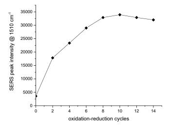
**Figure 7.** It shows the surface-enhanced Raman scattering (SERS) experiments results of 1  $\mu$ M Rhodamine 6 (R6G) solution measured by SERS chips with different oxidation-reduction cycles (0, 2, 4, 6, 8, 10, 12, and 14, respectively). It can be seen that in the first few cycles, the intensity of the SERS characteristic peak of R6G at 1510 cm<sup>-1</sup> increased rapidly and reached a plateau after 10 cycles.
