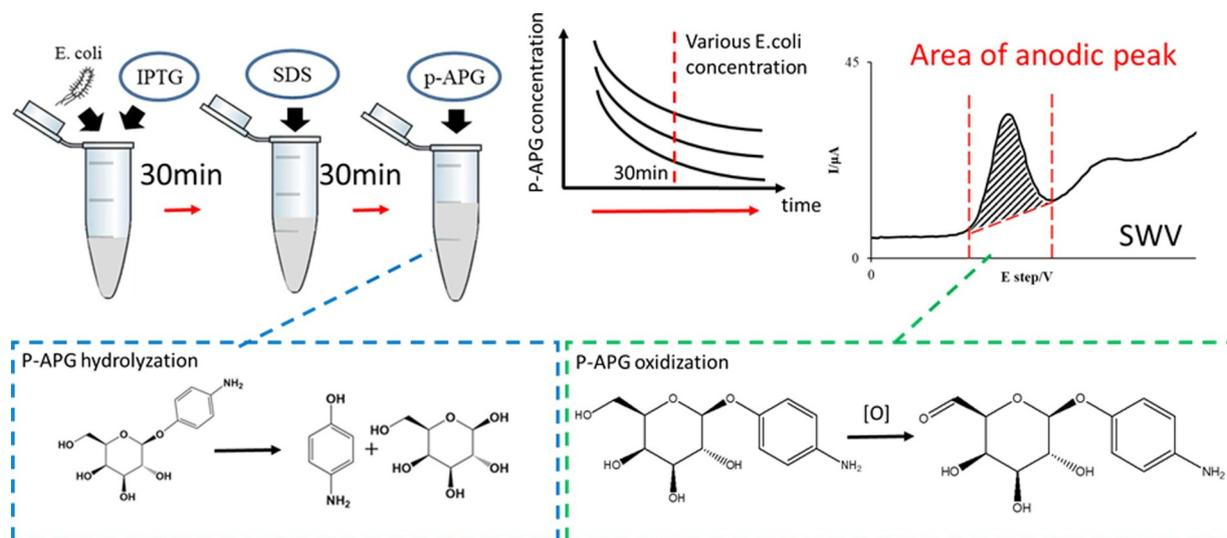
Fig. 1. Schematic of the experiments. *E. coli* was sequentially added IPTG, SDS, and p-APG, and the p-APG concentration, which is related to *E. coli* concentration, was determined by using voltammetry.
