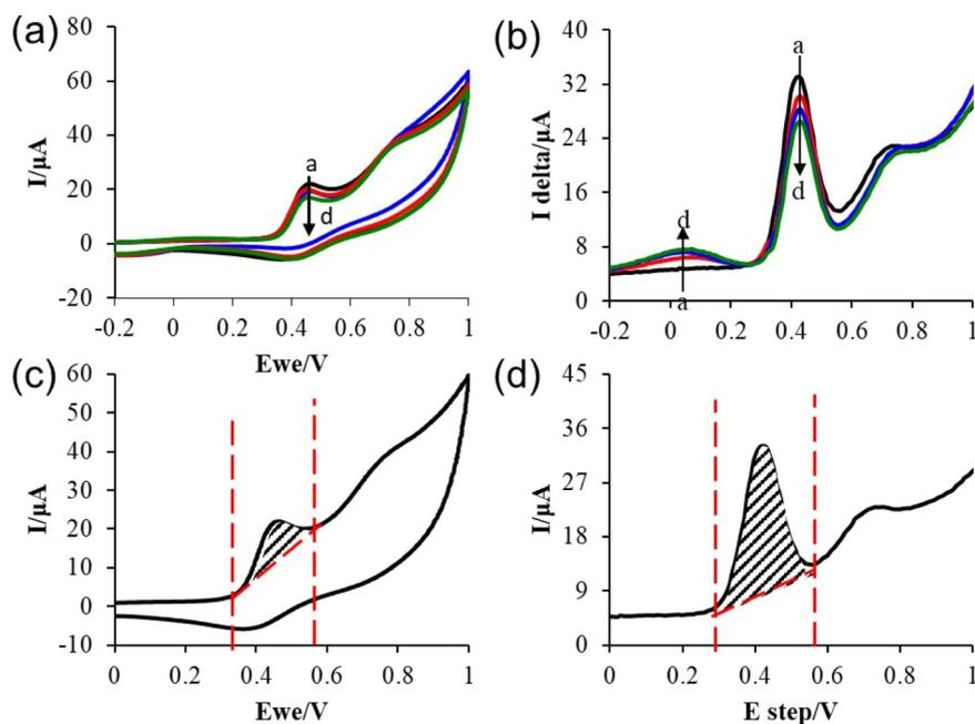
**Fig. 5.** After IPTG, SDS, and p-APG were sequentially added, with 30 min of incubation for each additive, the *E. coli* samples with concentrations 0,  $2.3 \times 10^2$ ,  $2.3 \times 10^3$ , and  $2.3 \times 10^4$  cfu/mL were measured using (a) CV and (b) SWV. *E. coli* concentration was quantified by calculating the area of anodic peak for (c) CV and (d) SWV.
