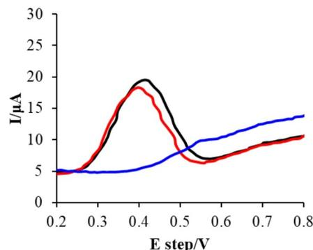
**Fig. 7.** Spiked sample testing by SWV method.  $I$ – $V$  curves of pure lake water (blue), p-APG added lake water (black), and  $10^2$  cfu/mL *E. coli* spiked lake water with adding IPTG, SDS, and p-APG (red). For interpretation of the references to color in this figure legend, the reader is referred to the web version of this article.
