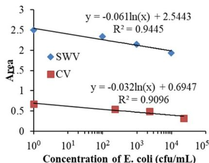
**Fig. 6.** Calculated areas of anodic peaks obtained using CV and SWV, showing a log-linear function of *E. coli* concentration. The slopes for the SWV and CV methods are  $-0.061$  and  $-0.032$ , respectively.
